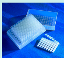
Figure B3: 96-well plate cluster tubes are composed of 8 (1.2ml) polypropylene tubes in strips that can be arranged in a 96-well rack
